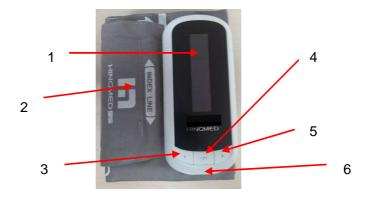
1 OLED screen; 2 Cuff; 3 Backward button; 4 Power on/off and Start/stop button; 5 Forward button; 6 USB port
